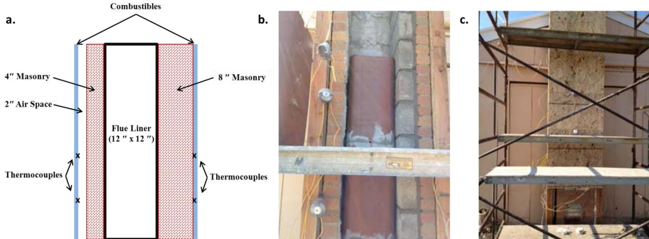
Figure 2 – (a) Diagram of the Chimney Test Configuration, (b) Photograph of the Test Chimney to Show the Masonry Configuration and (c) a Photograph Showing the Final Appearance after a Plywood Enclosure was Installed
