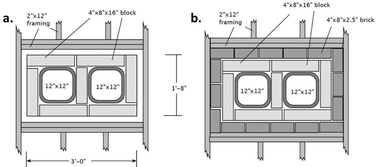
Figure 1 – Cross-sectional Diagram of (a) a Code-Compliant Chimney and (b) the Proposed Allowable Configuration
